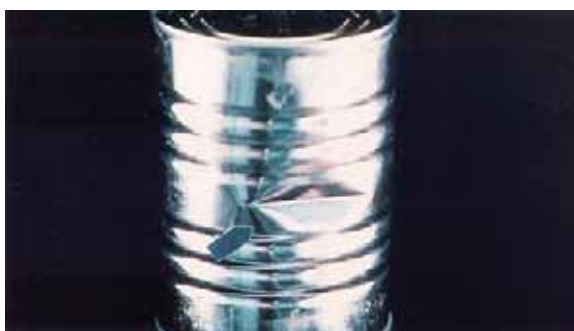
3 If the body dent does not significantly affect the side seam or double seams.
